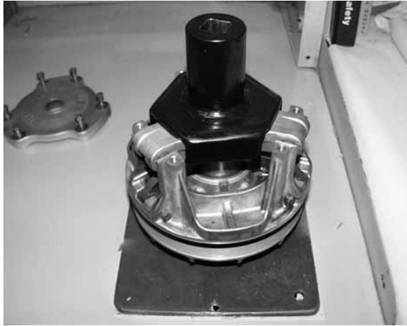
Clutch Holding Fixture: PN 2871358 Spider Removal Tool: PN 2870341
